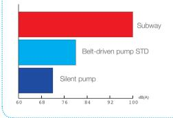
Thanks to the **flexible coupling transmission** and accurate machining of the **SILENT** vacuum units, the noise levels drop **below 72 dB (A)** compared to the 80 dB (A) of traditional belt-driven pumps.
